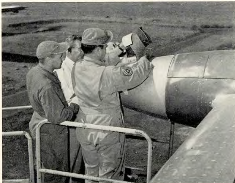
Outboard strip of reflective tape and cone of tape about trailing tip of heater pod serves two purposes.
