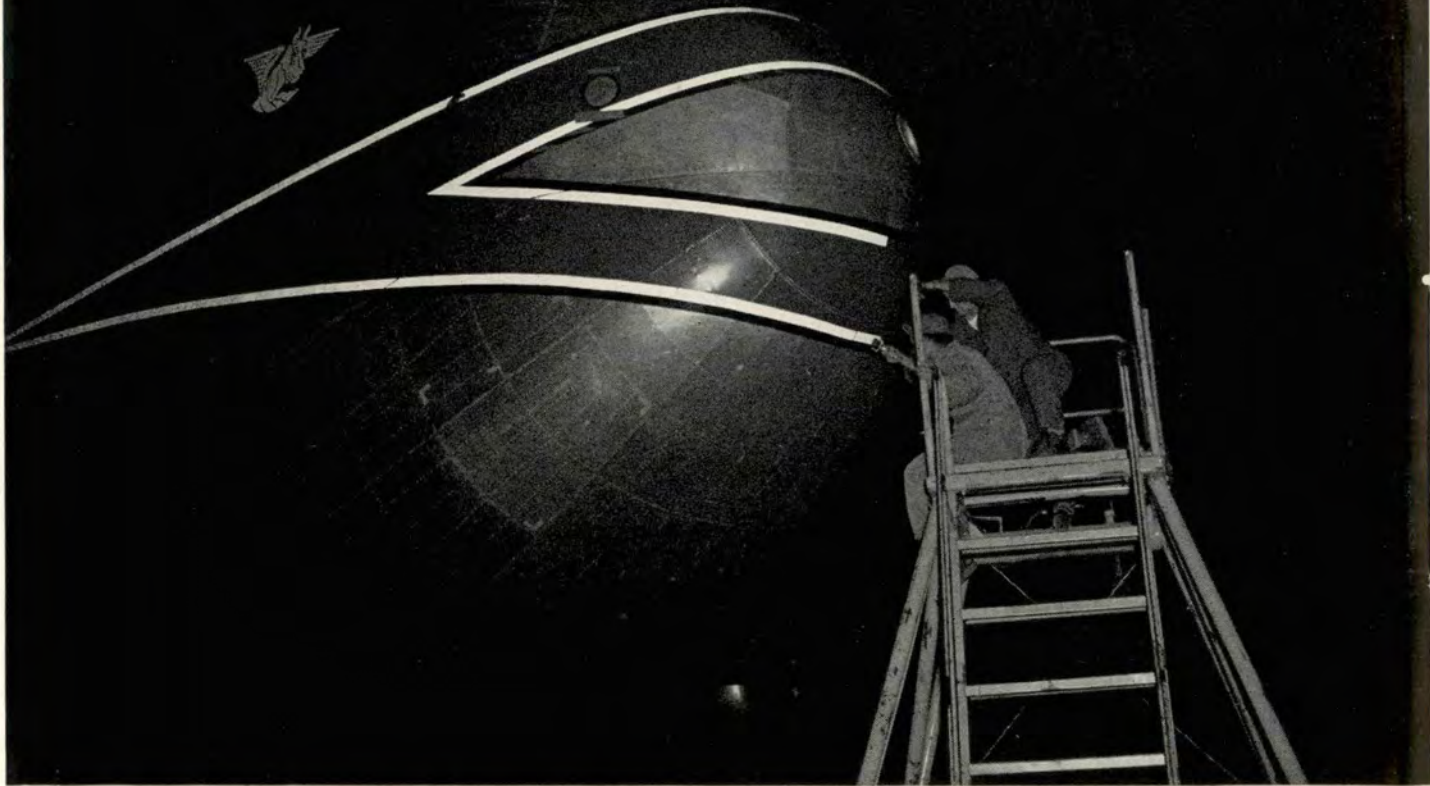
Crew chief fits band of reflective tape around the nose of a C-124. Material is self adhesive and flight tests prove that it will stand up better than paint. Lower photos: Taxiing aircraft are able to judge wing clearance and reflectors give reference point.
